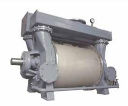
All of our liquid ring pumps handle wet or dry gases, with high tolerance to liquid carry over. The LR1B Series has an enhanced bearing design enabling reduced internal clearances for improved efficiency. Pumps are available in cast iron and 316 stainless steel construction as standard with other materials and corrosion-resistant coatings available. All are tested to DIN 28431:1987and are available as part of ATEX Category 1 and 2 T4 systems.
